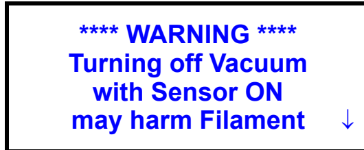
Figure 7-12 Shut down warning screens
